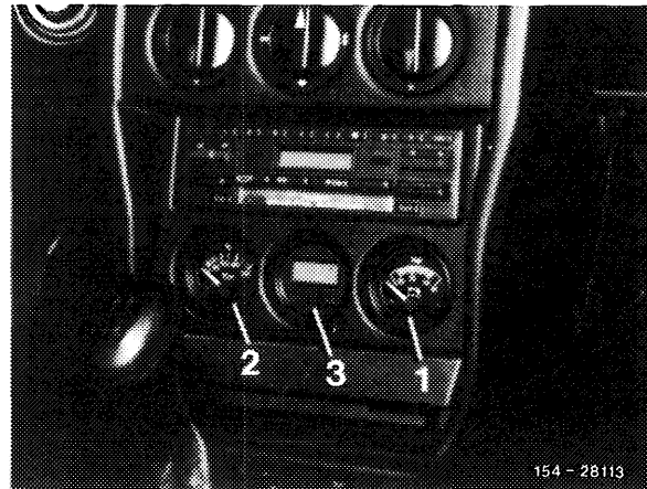
1 Voltmeter 2 Oil temperature indicator 3 Stop watch
