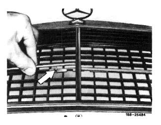
1 Energetically pull spring clip down with water pump pliers and turn to the left by  $90^{\circ}$ .
