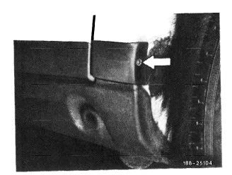
2 Unclip paneling by means of plastic wedge and remove.
