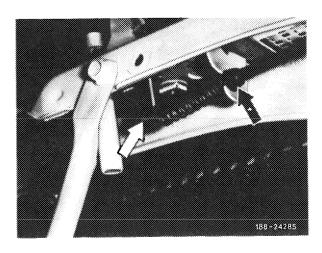
3 Unscrew screws on lock and remove lock.
