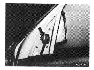
4 Unscrew fastening screws for outside rear view mirror and remove mirror.
