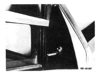
3 Unscrew screws and remove mirror.
