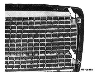
3 Unscrew screw at bottom of radiator shell.
