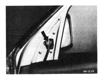
5 Unscrew fastening screws on electric motor.
