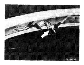
6 Press lock from pin on engine hood hinge on both sides.
