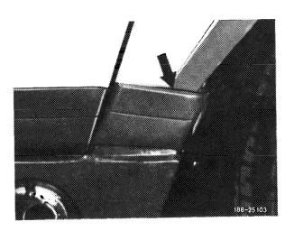
3 Unclip paneling by means of plastic wedge and remove.
