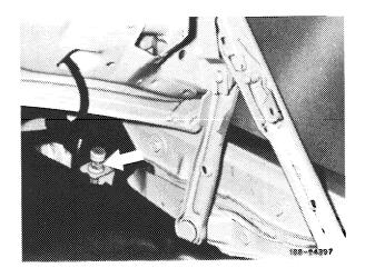
2 Loosen nut on lower threaded bolt.
