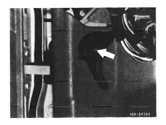
4 Remove rubber grommet on front wall pillar.
