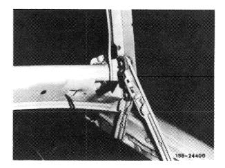
8 Mark position of lower threaded bolt left and right und unscrew nut.
