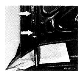
6 Adjust closing bracket on rear center piece for perfect opening and closing of trunk lid.
