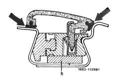
8 Align white plastic sectional elements in longitudinal direction in such a manner that they are not resting on the plug clamps.
