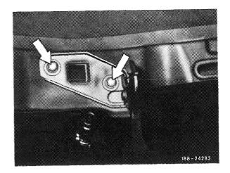
2 Fit engine hood. Air gap: a = 5 mm.
