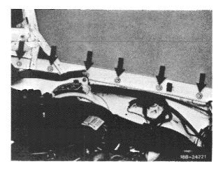
6 Unscrew screws in cutout of turnsignal lamp (flasher).
