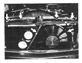
2 Disconnect hood cable control on holder and on lock.
