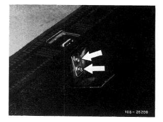
1 Unscrew screws and remove lock.
