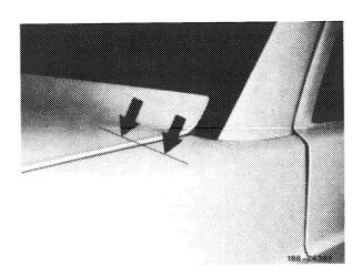
9 Set rubber buffers at the rear in upward direction until the engine hood rests at a light preload on rubber buffers, while paying attention to perfect fit between upper edge of engine hood and upper edge of front fender. Tighten counternut.
