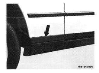
2 Unscrew screws on fender.
