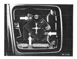
6 Tip mirror housing in forward direction and hold it in position. Turn electric plug connection by means of a suitable flat-jawed pliers in clock-wise direction and remove from holder.
