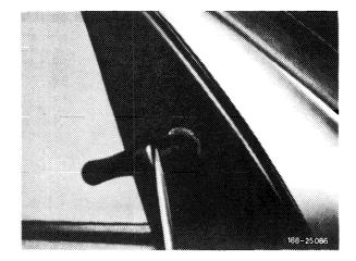
2 Unclip cover plate at top from door frame, pull in upward direction and disengage on inner door sheeting.
