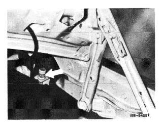
5 Loosen nuts on engine hood hinge in wheel house left and right.
