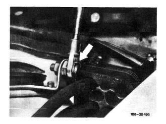
3 Pull off hose on check valve and release on holding clip.
