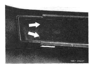
5 Push back detent on threaded holders left and right, simultaneously slide threaded holder in downward direction and remove.
