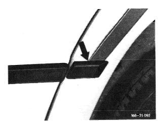
2 Press off protective strip rear by means of plastic wedge.
