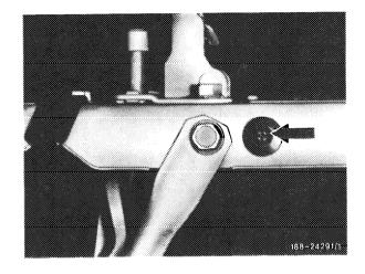
Note: On vehicles with air conditioning system, unscrew fan first (2 screws) when removing cover and then, after removing the 4 upper clips, swivel radiator to the rear.
