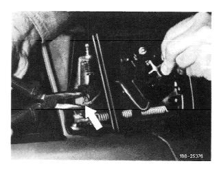
7 Pull electric connecting cable through mirror housing and completely remove electric motor.
