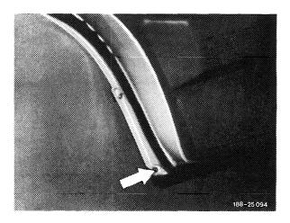
2 Unclip paneling by means of plastic wedge and remove.
