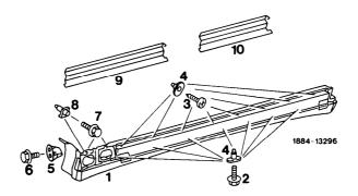
Panelling at wheelhouse front and rear removed Panelling at front and rear fender removed
