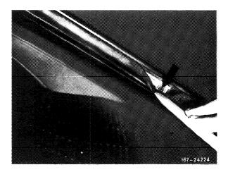
2 Press out rain strip, beginning at the front, in upward direction out of the 6 plug clamps and remove.
