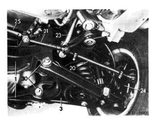
12 Lower pit lift approx. 50 mm and knock the rubber mounts out of their seats in the front axle carrier from below (see arrow).
