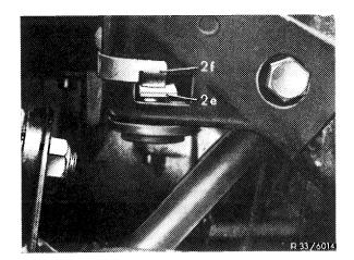
2e Fastening nut 2f Holder for fastening nut
