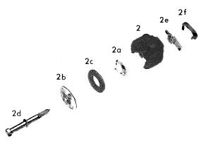
**Note:** For assembly of fastening nuts (2f) insert holder (2e) (if available).
