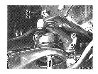
**Note:** On vehicles with longer wheelbase 3400 mm, models 114.008, 114.017, 115.103, 115.108, 115.112 and 115.119 there are washers (2g) between the front axle carrier and the rubber mount.
