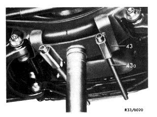
11 Loosen hex. head screws (2) of the four rubber mounts for front axle suspension on frame floor.
