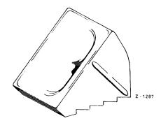
On level ground, protect one wheel of opposite vehicle end against moving off.
