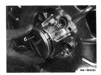
Plastic hub cap Holding cam Annular spring
