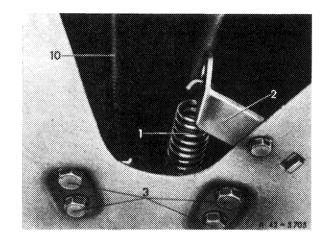
3 Unscrew adjusting screw (3) on adjusting bracket (1).
