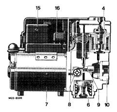
The hydraulic unit comprises three fast-switching solenoid valves. Of these valves, one each is associated with the lefthand or righthand front wheel brake and the third with the rear wheel brake.
