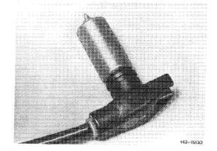
The speed sensors (34) for front axle are installed in steering knuckles.
