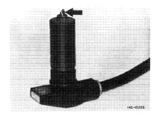
The speed sensors consist of a magnetic core and a coil. Rotation of toothed wheel or rotor, which is located at a given distance in relation to speed sensor, will change the magnetic field, so that an alternating voltage is induced in coil. This alternating voltage changes its frequency in accordance with the wheel speed and the number of teeth, i.e. the frequency is proportional to wheel speed.
