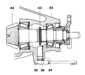
The speed sensor for the rear axle is single-edged (arrow) and has a diameter of 15 mm.
