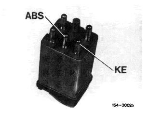
Version with CIS-E injection system starting September 1985 (5 pins)
