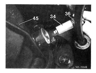
7 Attach rpm sensor with hex. socket screw (35) to rear axle housing. Tightening torque 8 Nm.
