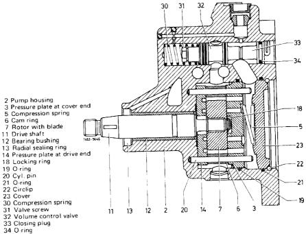
22 Check drive shaft (11) and bearing bushing (12) for wear. If required, install bushing from repair set "drive shaft".
