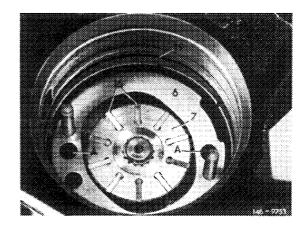
24 Check ground surfaces of volume control valve (32) and bore in pump housing for wear and damage. If the sliding surfaces are showing score marks, renew complete power steering pump. Never replace volume control valve only.
