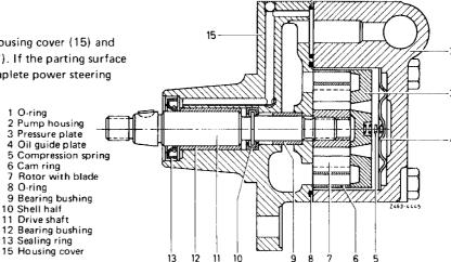
17 Check end play of drive shaft (11), which is max. 0.7 mm on a new pump and should not exceed 1 mm on a used pump.
