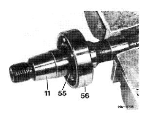
17 Knock needle bearing out of housing by means of a suitable mandrel.
