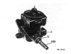
13 Screw back hex. screw of puller (050) and slip device on drive shaft, while punching with claws (051) through sealing lips of radial sealing ring (13).
