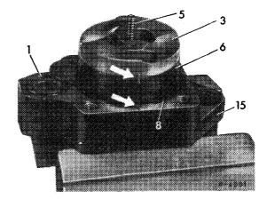
5 Remove thrust plate (3) from set pins, then remove cam ring (6).
