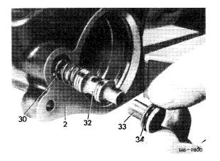
Light alloy power steering pump 2 Pump housing
