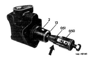
14 Turn clamping cone (arrow) of puller (050) to the right up to stop and pull sealing ring out of housing.
