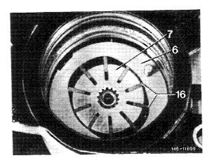
13 Remove O-ring and cam ring (6).
