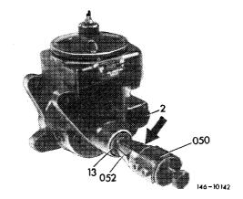
9 Turn clamping cone (arrow) of puller to the right up to stop, then pull sealing ring out of housing.
