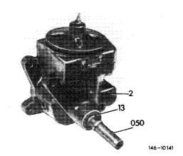
8 Turn hex. screw of puller (050) back and slip device on drive shaft, while punching through lips of radial sealing ring (13) by means of claws (052).
