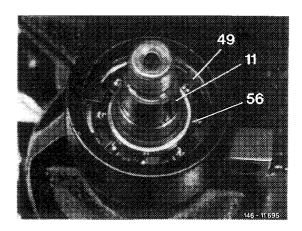
15 Press drive shaft out of housing.
