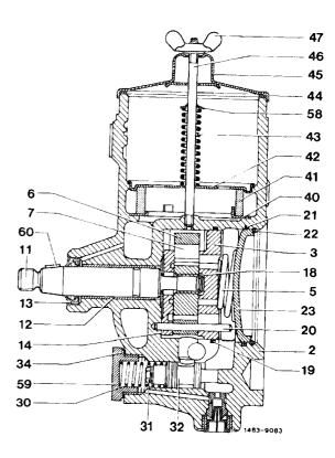
19 On light alloy power steering pump, unscrew closing plug (59) from housing, remove compression spring (30) and volume control valve.
