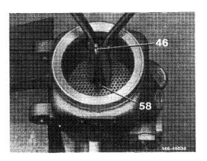
5 On light alloy pump 1st version, take steadying basket (60) out of pump housing.
