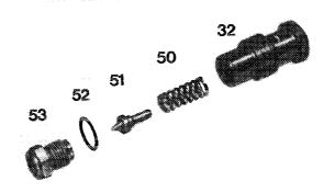
Pressure relief valve 2nd version with valve cone
