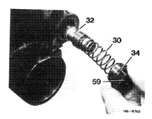
20 Clamp volume control valve (32) of both pump versions with its unground part into vise and unscrew valve screw (53) of pressure relief valve. Make sure that no spacing washer (52) is lost. Remove valve cone (51) and compression spring (50) from volume control valve.
