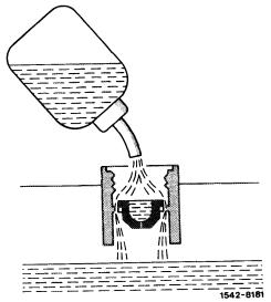
The distilled water flows through circularly located slots (4) into cell. The air displaced from cell flows through 4 vent bores (3) into the open air.
