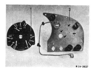
4 The indicating instrument can be removed after loosening screws and nuts from switch plate.
