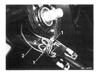
5 Pull off 14-point plug (arrow) and remove combination switch.
