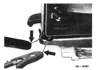
**Note:** Adhesive material which is visibly pushed-out at linings can be cut off with a moistened industrial knife.
