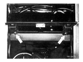
10 Remove screws on the forward end of the footwell, LH and RH sides.
