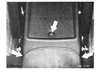
15 Lift up center console at rear end and pull to the rear by approx. 90 mm. In doing this, pull outward the lateral sections of the covering in the region and rest them on the cross member.
