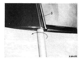
**5** Pull trimstrip (3) out of remaining clips starting from below and using the plastic wedge.
