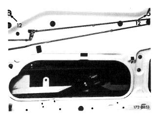
**4** Crank window up until guide bracket (6) and front edge of pane are in alignment.
