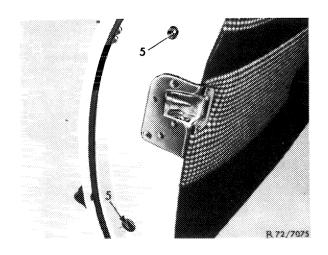
**Note:** Adjust lateral preload of pane by means of screws (5) and nuts (10).
