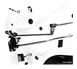
**13** Following adjustments, lubricate all slide surfaces on window guide rails with anti-corrosion grease Part No. 000 989 31 51.
