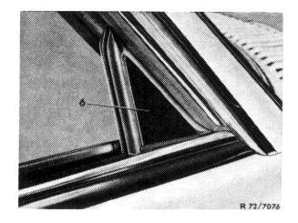
For this purpose, loosen both screws (4) on guide bracket (6) front.
