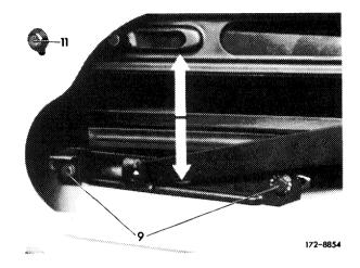
**5** Adjust pane by means of the two front screws (17) in such a manner that pane rests against front sealing rubber at moderate pressure when door is closed.
