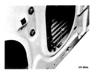
**Note:** When preload is correctly adjusted, the front upper edge of opened window will just touch rubber seal when door engages in first stage of door lock. With the door completely closed, pane (2) should now rest in its complete length against inner lip of front rubber seal (1),
