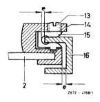
For this purpose, screw both threaded studs (13) on front slide piece completely down, then screw threaded studs (13) back for approx. one 3/4 turn.
