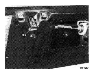
12 Attach holding spring (15) to vacuum element (5) and screw to lefthand cover of rear center piece (29) by means of oval head screws.
