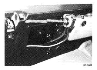
11 Introduce vacuum element into rear center piece, attach control rod and secure with locking ring (33).
