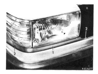
2 Loosen all three fastening screws (5). Push light unit slightly downwards and swivel in outward direction.
