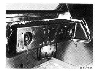
2 Unscrew fastening nuts (1). Remove housing in inward direction, light window with gasket in outward direction.
