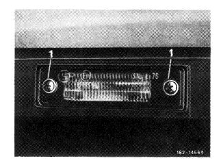
4 Pull cable with coupling inwards upon removal of rubber grommet (1). Remove righthand and lefthand license plate lamp from inside.
