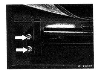
6 Unscrew forward screw of seat guid rail on both sides.
