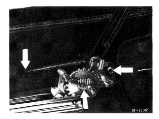
6 Screw out of the tunnel the screw of the connecting tube mount.
