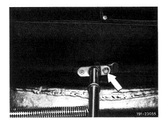
7 Turn screw of mount out of side member and take out connecting tube.
