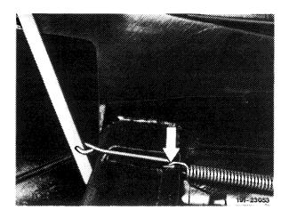
4 Remove lock from forward end of connecting rod and detach the latter.
