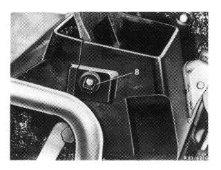
6 Insert sealing strips (4) into heater box bottom.
