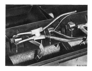
3 Pull the two clips (2) with circlip pliers off in direction of arrow and remove shim (3).
