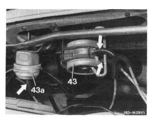
43 Double-acting vacuum element 43a Single-acting vacuum element
