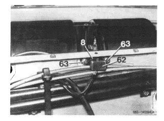
8 Ambient temperature sensor 62 Electric plug 63 Screw
