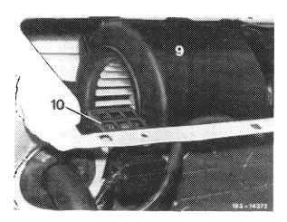
3 Unscrew two screws (arrow) on pre-resistor (10) and remove pre-resistor from front wall.
