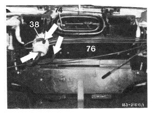
19 Mount air duct-center with four clamps (arrow) on heater box.
