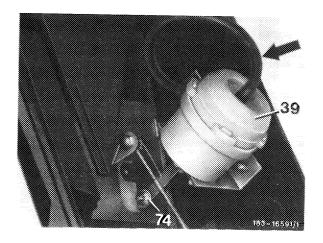
14 Mount air duct-center with four clamps (arrow) on heater box.
