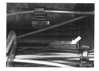
9 Remove clamping springs (arrow) by means of pliers for locking rings from air conditioning cabinet top and scoop.
