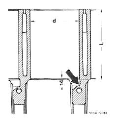
2 Cut the lower protrusion of the bronze strip on the main guide shoe (arrow) as the recess at the bottom of the cylinders allows only approx. 14 mm protrusion of the honing stone.
