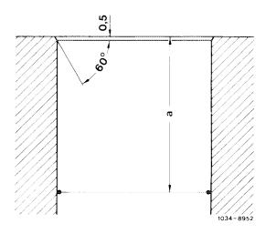
15 For chamfering, use a suitable hand milling tool with an angle according to the above drawing.
