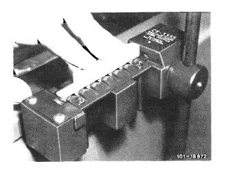
23 Set up the cylinder diameter by means of the setting gauge.
