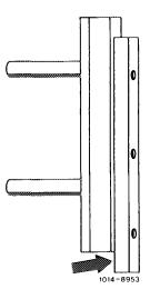
3 The specified stone sets of 89 mm length must be shortened to 70 mm. To do so, cut the honing stone at the top (not the holder) using a metal saw.
