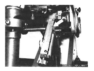
7 Adjust stone projection (arrow) with the gauge according to the table.
