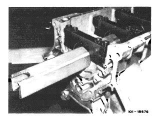
6 Adjust stroke (cylinder length) on the stroke scale according to the table "Prehoning".
