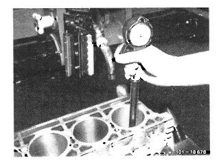
21 Clean cylinder walls with filtered honing oil to remove all silicon particles and to avoid scratches during the subsequent silicon-lapping process.
