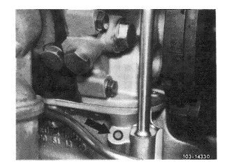
Do not mix up oil dipstick guide tubes during assembly jobs, since otherwise wrong oil levels will be indicated.
