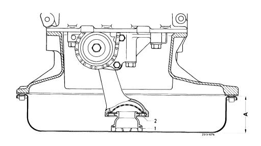
As a spare part, oil pans are supplied with 2 bores for oil dip stick guide tube. Close bore which is not required with a closing plug (arrow).
