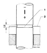
b) Plus deviation (+) is indicated when the measuring edge (2) is above the red measuring groove (1).
