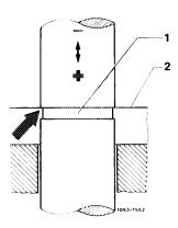
c) Minus deviation (—) is indicated when the measuring edge (2) is below the red measuring groove (1).
