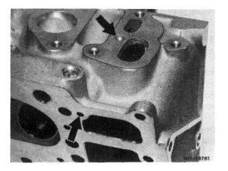
Since December 1974, the installed chain tensioner is provided with a venting bore for defoaming of the oil.
