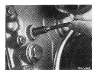
6 Remove tensioning rail.
