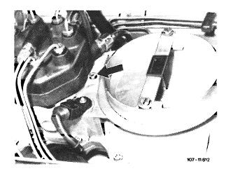
Insert screw driver through bore into socket on idle speed mixture control screw and adjust emission value by turning.
