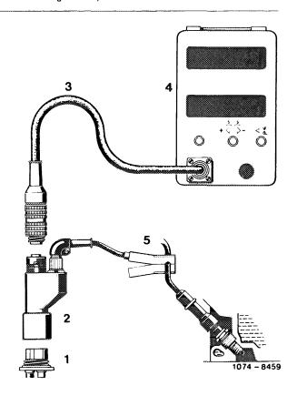
5 Check-intake system for leaks. For this purpose, spray all seal points with Iso-Oktan DIN 51756 or benzine.
