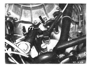
10 Adjust idle speed emission value. For this purpose, unscrew closing plug (arrow).
