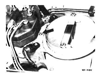
Insert allen wrench through bore into socket of idle speed mixture regulating screw and set emission value by turning screw.
