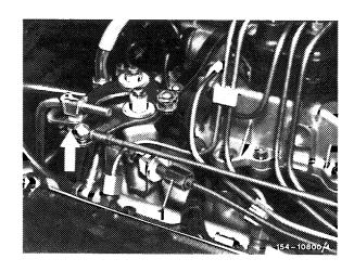
7 Check whether roller (3) in gate lever (4) rests free of tension against end stop. Adjust by means of connecting rod (2), if required.
