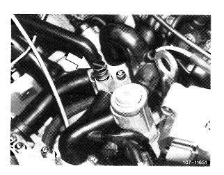
9 Adjust idle speed emission value. For this purpose, unscrew closing plug (arrow).
