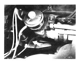
5 Check intake system for leaks. For this purpose, spray all sealed points with Iso-Oktan DIN 51756 or benzine.
