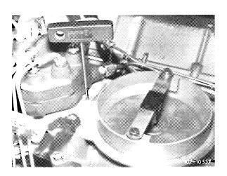
Following adjustment, on vehicles manufactured after October 1, 1976, install a blue safety plug (arrow) MB-part no. 000 997 56 86.
