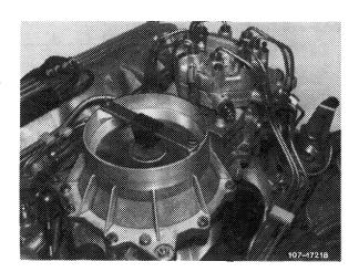
4 Connect connecting lines of quantity reference measuring unit to fuel distributor (sequence according to Fig.) and plug fuel return line into filler neck of fuel tank.
