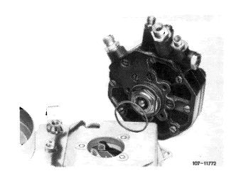
9 Check adjusting lever (1) in air flow sensor and control piston (2) in fuel distributor for easy operation.
