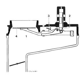
10 Check association of control piston in relation to air flow sensor plate and adjust, if required. For this purpose, switch on ignition and pull cable plug from safety switch. The fuel should now just stop to flow at outlet connection for injection lines. Adjust association by means of idle speed mixture control screw, if required.
