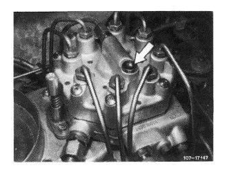
The pressure compensating valve is closed as long as fuel system is under pressure.
