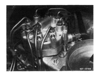
In addition, the fuel distributor top has a pressure compensating valve (arrow), as well as a compression spring which is integrated above control piston.
