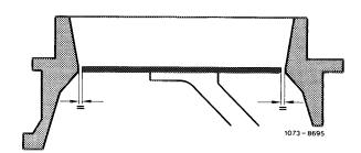
7 Tighten fastening screws to 5.0-5.5 Nm.
