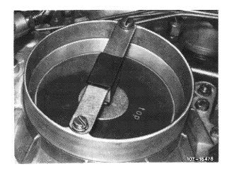
3 Heat fastening screw with a hot air blower and screw out carefully (risk of tearing).
