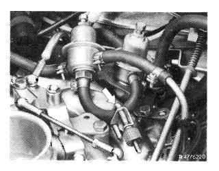
c) Check ball valve in pressure connection of fuel pump by switching-on ignition while disconnecting (pinching) fuel hose of fuel feed line in front of ring line (arrow) the moment the fuel pump stops.
