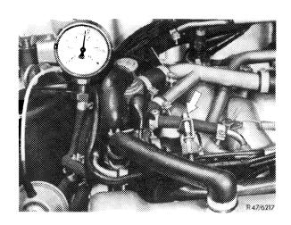
b) Check with pressure regulator by switching-on ignition and disconnecting (pinching) fuel return hose, behind pressure regulator (arrow) the moment the fuel pump stops.
