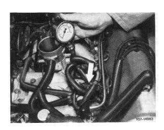
4 Run engine at idle speed, check fuel pressure.
