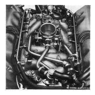
5 Renew defective injection valves. For this purpose, loosen hose clip on ring line and remove locking ring (4) from fastener (2).
