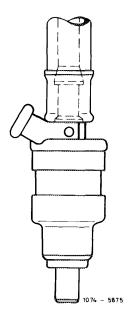
Former injection valve Hose sleeve: height 17 mm
