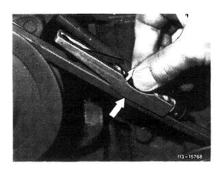
5 Read adjusting value on point of intersection of indicator arm and upper scale (KG-scale, arrow).
