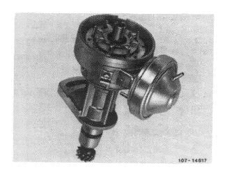
4 Remove vacuum box while lifting box slightly so that the pull rod (1) comes out of bolt (2) of pole disc (3).
