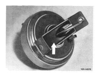
6 Introduce vacuum box in such a manner that the pull rod (1) engages on bolt (2) of pole disc (3).
