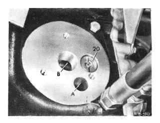
Bypass valve filter element Valve 20
