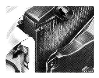
6 Lift-out radiator with air-oil cooler in upward direction.
