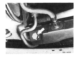
5 Push holding springs in direction of arrow or push rubber loops out of holder.
