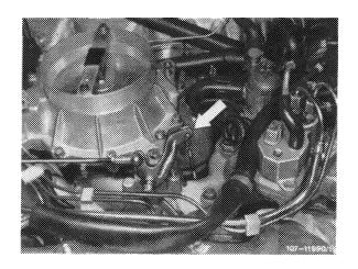
3 Vehicles with cruise control/tempomat. Check whether bowden wire for cruise control/tempomat rests free of tension against regulating lever. Adjust with adjusting screw (1), if required.
