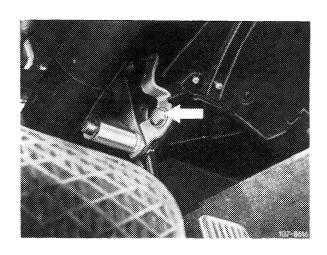
6 Adjust control pressure rod (at idle speed position). For this purpose, compress adjusting clip (7) with pliers and push control pressure rod completely to the rear against stop.
