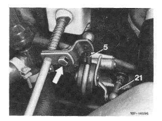
If full throttle or idle speed stop is not attained with this adjustment, set pushrod (5) from longitudinal regulating shaft to accelerator pedal to specified length, measured from center of ball socket to center of damping ring.
