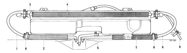
Fuel expansion tank with 5 connections
