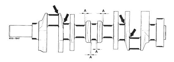
The running surface for the rear radial sealing ring is hardened and ground without helix (previously  $60^{\circ}$  helix).
