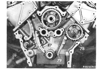
78 Intermediate gear for distributor drive
