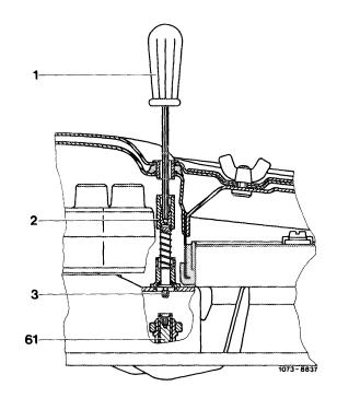
After each adjustment, depress accelerator pedal briefly and test for variations between 2500 rpm and idle speed; reset if necessary.
