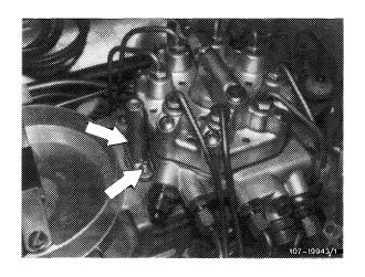
Install new repair kit, Part No. 102 070 01 74 by tightening bolts until head shears off.
