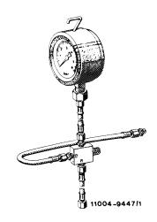
Connection A = Hose line to fuel distributor - lower chamber
