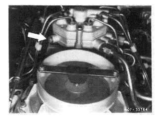
2 Connect hose line from connection "A" to bottom chamber.
